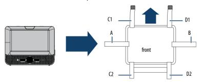
2 Slide the horizontal straps A and B through the slots on the back of the DVD player or monitor, then fold and secure them on to the back of the mounting plate until the Velcro attaches.
